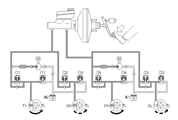
Electronic brake force distribution (EBD) is integrated in the ABS system and controls the braking forces to the rear wheel brakes. Electronic brake force distribution (EBD) replaces the relief valve, which otherwise reduces the pressure in the brake circuit for the rear wheels and prevents premature activation of rear ABS control.
