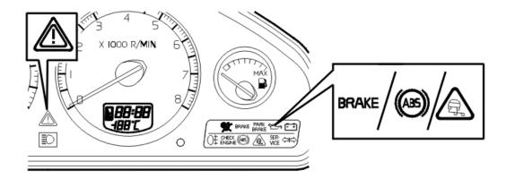
The brake system uses four warning lamps positioned in the combined instrument panel.
