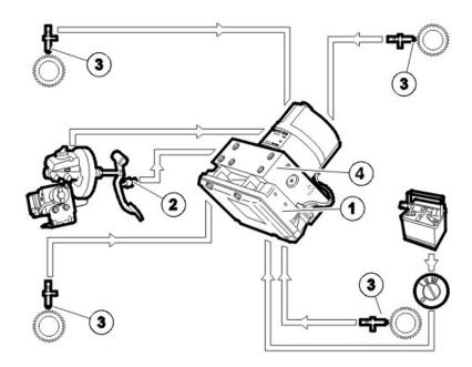
While driving, the brake control module (BCM) (1) registers the acceleration and deceleration of the wheels. The 4 wheel sensors (3) (one on each wheel) give the brake control module (BCM) information about the rotation speed of the wheels. The brake control module (BCM) calculates the speed of the car using this information and puts it out on the Control area network (CAN). There the signal is accessible for other systems.
