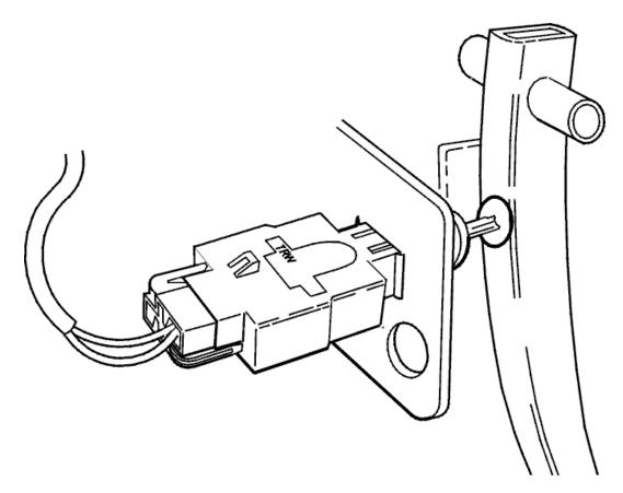
The brake lamp switch is a single pole switch positioned at the brake pedal lever. The brake lamp switch self-adjusts during installation.
