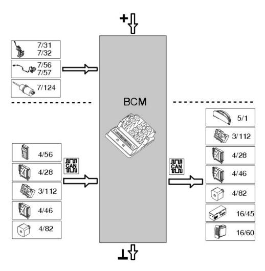
Signals, Brake control modules (BCM) with DSTC (dynamic stability and traction control)
