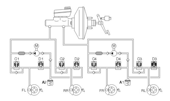
When the driver is not braking, the brake system is unaffected (i.e. the master cylinder is in the rest position and the connections between the brake fluid reservoir and the rest of the hydraulic system is open). There is no pressure in the system. In the ABS hydraulic modulator valve block, the hydraulic valves are in their rest position. In other words, the inlet valves are open and the outlet valves closed.
