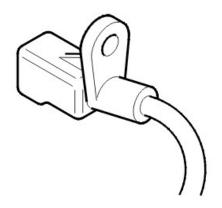
There are four wheel sensors, one at each wheel. The wheel sensors supply the control module with information about the rotation speed, acceleration and retardation of each wheel. By recording the pulses, the control module can calculate the wheel speed.
