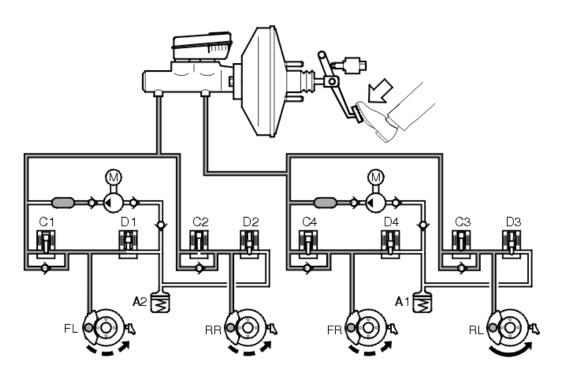
When a wheel locks-up under braking, the brake control module (BCM) begins to close the inlet valve for the relevant brake circuit so that the supply of brake fluid from the master cylinder is interrupted. This means that the hydraulic pressure cannot increase irrespective of the pressure in the master cylinder (constant pressure, see the right-hand front wheel - FR). The hydraulic pump starts at the same time.
