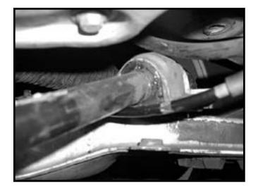
Make a note how the bar is fit onto the subframe. It is important to orient the new bar correctly to clear the steering arms etc.
