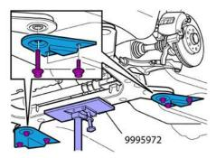
Lower the sub frame at the rear edge carefully, check that the steering gear pins release from the sub frame and that the bracket to the exhaust pipe is free for the brake pipe.
