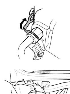
Remove the lock grip pliers from the feeder hose.
